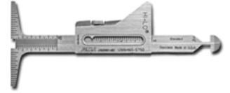
HI-LO Welding Gauge Measures Internal misalignment, Fit-up gap, Bevel on end preparation, Crown height, Pipe wall thickness and Fillet weld size
