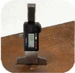
The PG-1 is a Pit Gauge based on a direct reading digital vernier caliper. The PG-1 is easy to use and provides fast and accurate measurements of surface pits, gouges, dents, undercut etc. The PG-1 is made in hardened stainless steel and its 0.5mm (0.02") diameter probe will access even the smallest pits.
