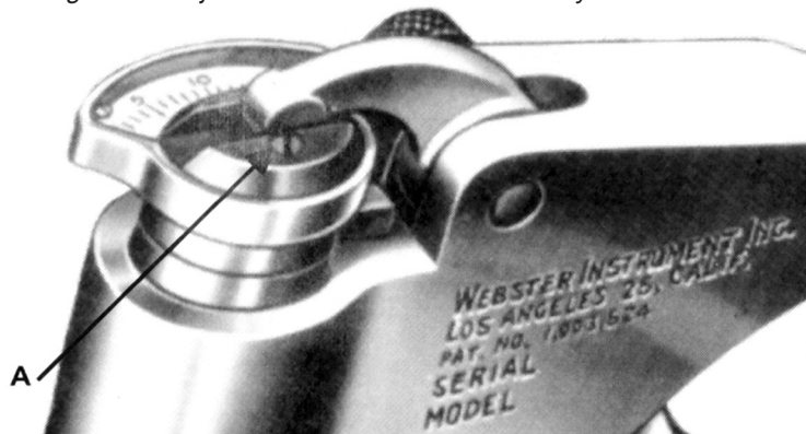
Fig 2 Zero adjustment screw "A" is indicated by arrow
