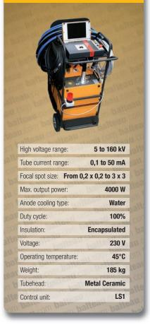
The XMD160/4KW gives the flexibility of a mobile unit and and is as powerful, stable and sturdy as a stationary unit. It gives you more flexibility than a portable unit in places where room for the tubehead is reduced.
