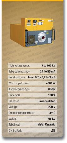
Introducing the Baltograph series, the XSD160 is the first unit of a complete set based on a solid insulation HV module.
