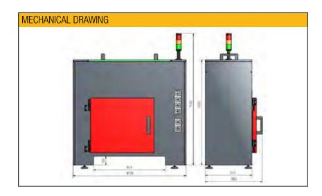
These cabinets are generally made of a steel structure with lead reinforcement to assure a proper shielding against radiation outside of the confined area («sandwich» type assembly: steel-lead-steel). This user-friendly equipment can be very easily operated with a maximum safety.
