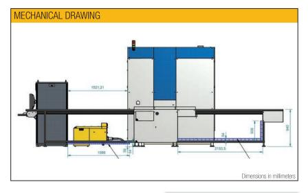
Composed of a shielded cabinet, a manipulator, conveyors In & out, an x-ray generator and tubehead from 160kV to 225kV, a flat panel & much more, the AIS500 is the answer to any business who wants to inspection their components from their production line at any stages of the manufacturing.
