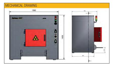
This shielded cabinet made of a steel structure with lead reinforcement ("sandwich" type assembly : steel-lead-steel) includes a directional constant potential generator of 160 kV or 225 kV as well as a flat panel. The AIS958 is associated with our «Inspection Suite» of softwares, including our image processing software IPS012.
