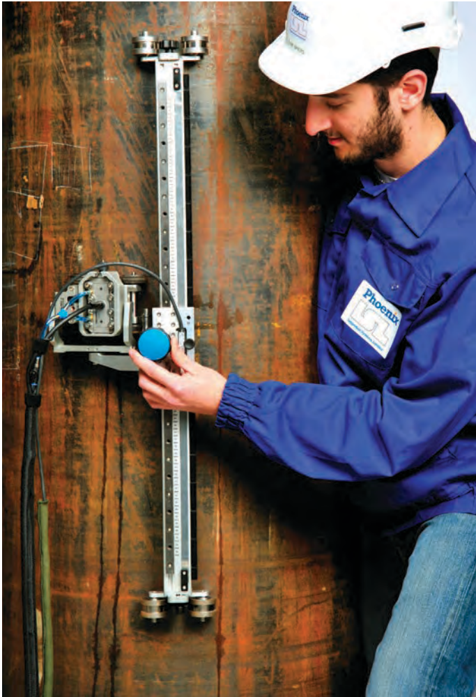
MapMan performing corrosion scans on 24" OD pipe
