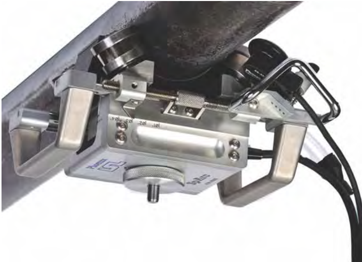
Sp-Arc inspecting the underside of a 3" pipe
