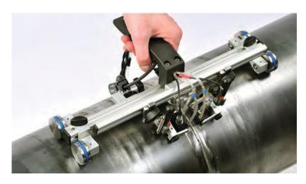
Swift is a compact single axis, magnetic wheeled scanner that holds a pair of probes for weld inspection. This low profile scanner operates on 3" pipe (Ø88.9mm) up to flat. Swift has the innovative option of pivoting wheel units to enable B or D scans.
