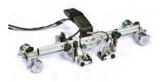
Dual direction Swift, with optional pivoting wheel units, for B scans with two TOFD probes
