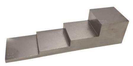
**AS2083 Block 7** (also known as **Step Wedge**) is an ultrasonic testing (UT) tool used for the calibration of 0° (normal) longitudinal transducers. Material of varying thickness for calculating Time base (Range), and Velocity.
