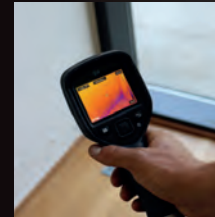
Find air infiltration problems
