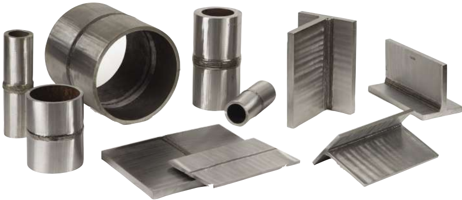
A selection of advanced weld flaw evaluation specimens
