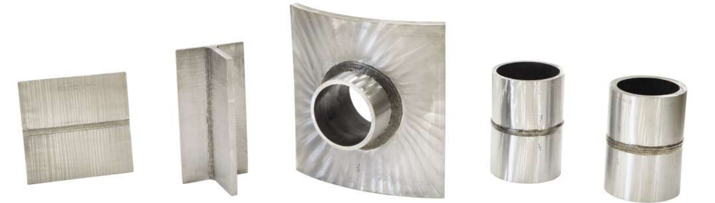
An example of some ultrasonic specimens
