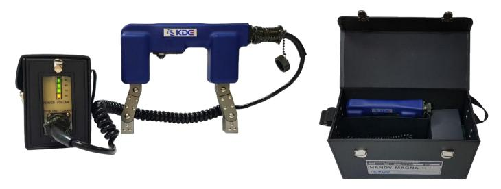
The MP-A2D uses a DC 12V battery to provide the unit with a mobile power supply, making the unit portability, and ideal for use in areas that do not have mains power supply.
