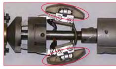
The *picture above* shows the white BFET sensors in a retracted state. The sensors are circled in red.
