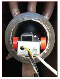
**TesTex manufactures a wide variety of probes, scanners and accessories to complement our systems.** These items range from High Frequency Eddy Current probes to Low Frequency pipeline scanners.
