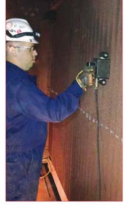
developed Low Frequency Electromagnetic Technique (LFET) scanner designed to detect flaws in the tube from the O.D. (pictured above). The LFET scanner is able to detect, and quantify flaws in the tubes even through the fins. This allows us to look for pitting and general wall losses like flow accelerated corrosion.
