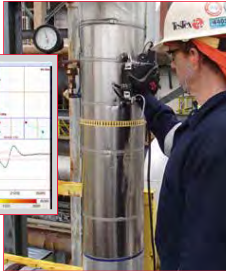
Waveform shows two pits 30% and 60% (blue circles) and a weld (red circle)
