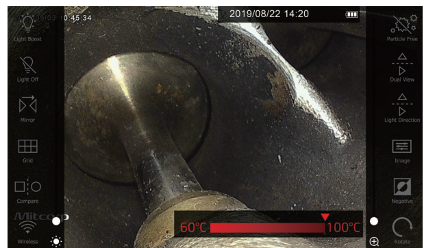
3 stage temperature warming & auto shut down function
