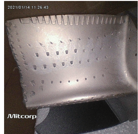
1600*1600 output by 3.9 mm HD probe (30 mm distance)
