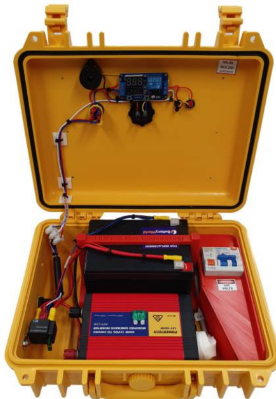
Figure 3 For transit and freight remove Red and Black battery cables by grasping the yellow spade terminals and removing from the battery. The shroud shown on the righthand side covers both GPO and RCD. The revised battery clamp secures the battery in 3 axes.
