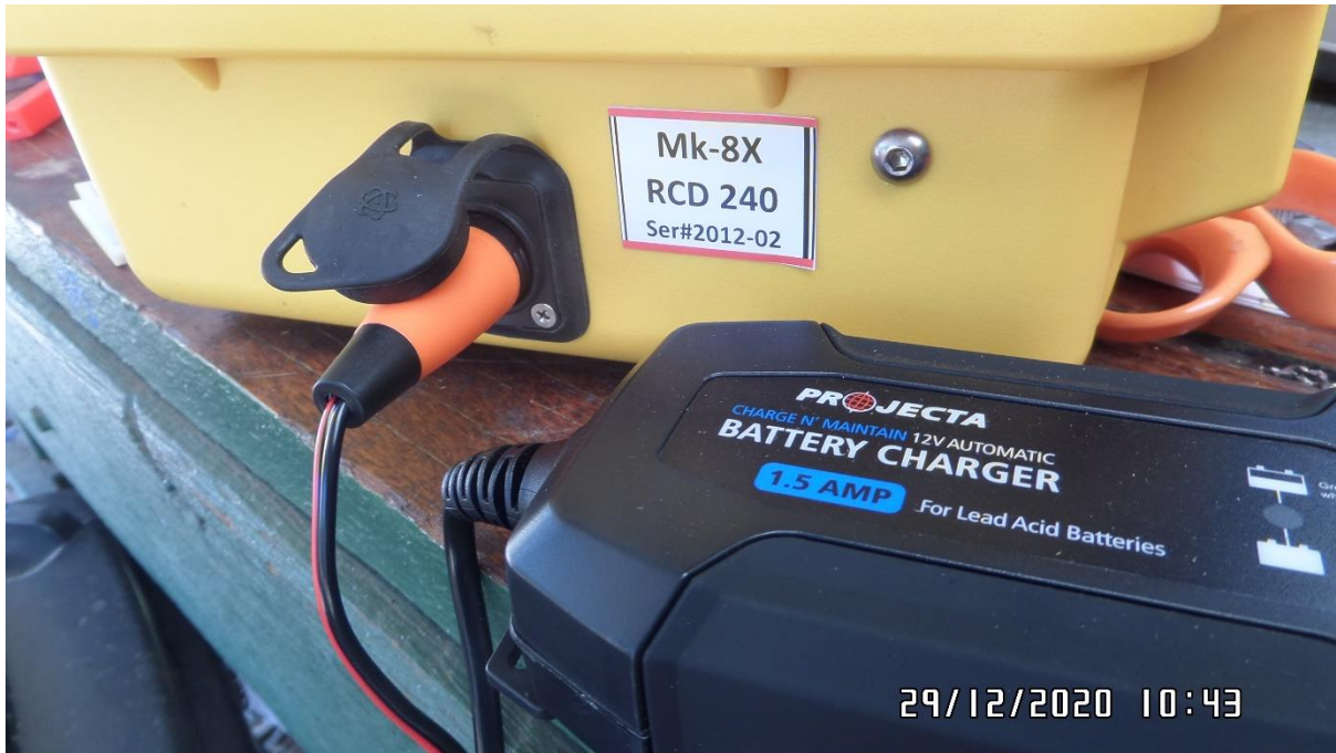
Figure 4. Projecta AC015 charger and XLR 3-pin charge plug replaces earlier model AC150 and 2.5mm charger plug.
