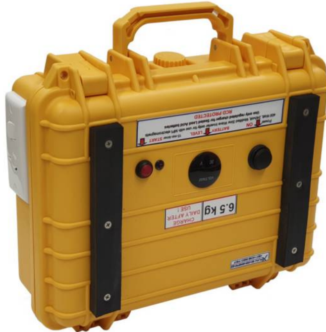
Figure 2. Mk-8X-RCD MPI Inverter. The 2.5 mm charging plug used in previous models has been replaced with a 3-pin plastic XLR to remove the chance of an OLYMPUS 24-volt Li-Ion power supply being inadvertently used.
