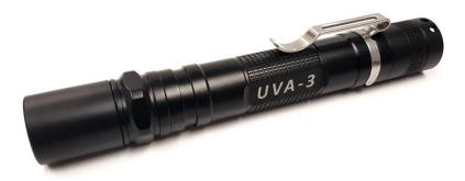
The UVA-3 is a hand-held battery powered Ultraviolet inspection lamp used for a range of NDT applications. The filtered 365nm output makes it ideal for Fluorescent Magnetic Particle Inspection (MPI), and Fluorescent Dye Penetrant Inspection (DPI), as well as leak detection applications when used with a suitable additive (such as Spectroline Oil-Glo).
