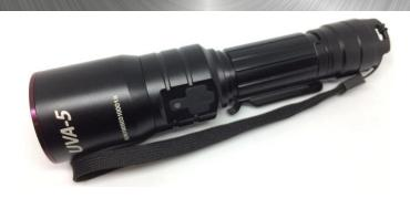
The UVA-5 is a hand-held battery powered Ultraviolet inspection lamp used for a range of NDT applications. The filtered 365nm output makes it ideal for Fluorescent Magnetic Particle Inspection (MPI), and Fluorescent Dye Penetrant Inspection (DPI), as well as leak detection applications when used with a suitable additive (such as Spectroline Oil-Glo).
