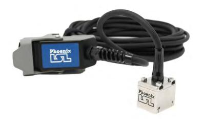
High performance linear phased array probes, designed with piezo-composite elements to provide high resolution imaging and to maximise sensitivity.
