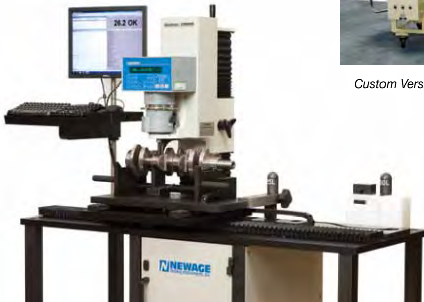
Custom Versitron® Test System for automotive crankshafts.
