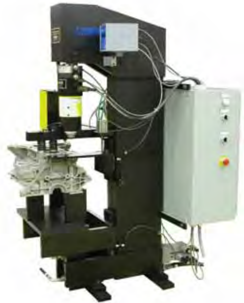
Custom Automatic Brinell for automotive engine blocks.
