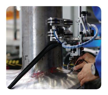
NozzleScan is a versatile, low-profile manual scanning solution developed for the inspection of nozzle welds in both setthrough and set-on configurations, with the option of a motorised version for automated inspection.
