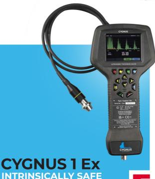
The Cygnus 1 Ex Ultrasonic Thickness Gauge is a rugged, handheld, intrinsically safe instrument designed for taking reliable thickness measurements in Zone 0 Explosive Atmospheres. It features a large colour LCD display and 3 measuring modes for through-coat measurements and various materials - including heavily corroded metals. Although designed for ease of use, the gauge boasts advanced datalogging and manual measurement mode.
